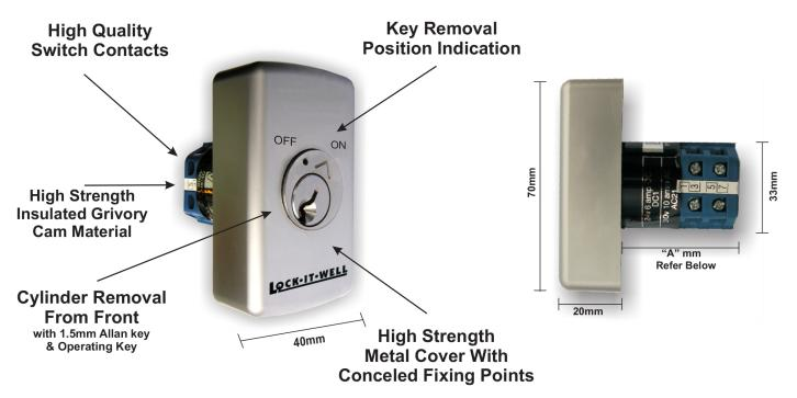
Designed for control of Automatic doors on commerical building (Can be used for other applications). The "A" series uses a unique removable cylinder enabling convenient master keying and key recombinations. The lock cylinder also serves to lock in place a metal cover protecting the mounting screws from removal.
